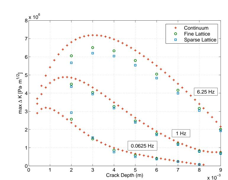
The figure shows the maximum [effective]  $\Delta K_I$  values for the thermally striped continuum and the two lattices at three striping frequencies: 0.0625Hz, 1Hz and 6.25Hz. The continuum curves show similar behaviour to that observed in earlier works, with the local maxima of  $\Delta K_I$  increasing and shifting further to the right for lower frequencies. For sufficiently long cracks, the lattice curves exhibit the same qualitative behaviour as the continuum.
